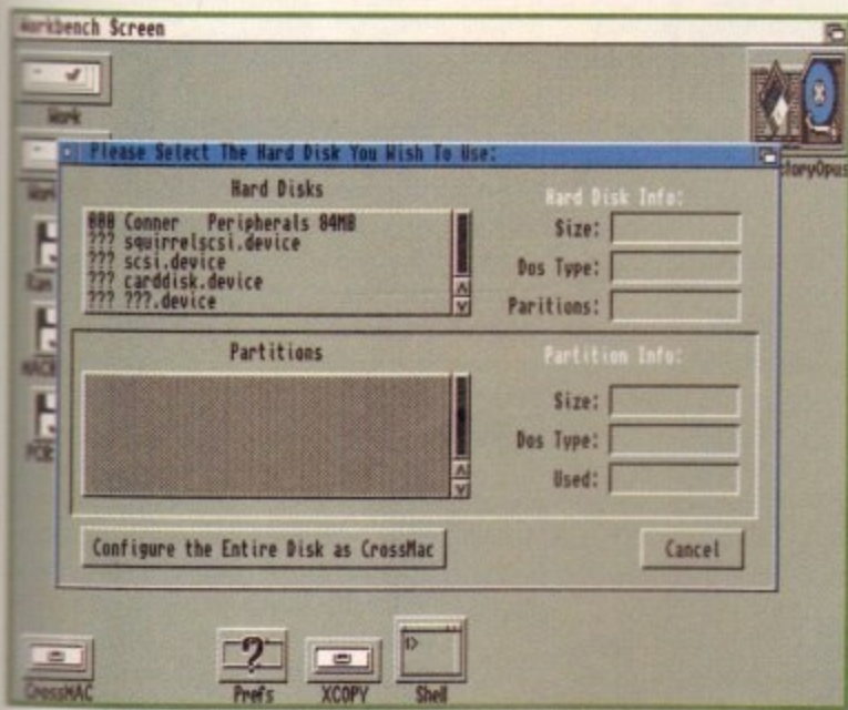
Any hard drives attached to your Amiga can be configured for use as either a 'real' Mac hard drive or a simulated one using CrossMac
